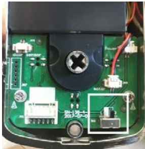
L or R Toggle Switch – Bottom Right Hand Corner
